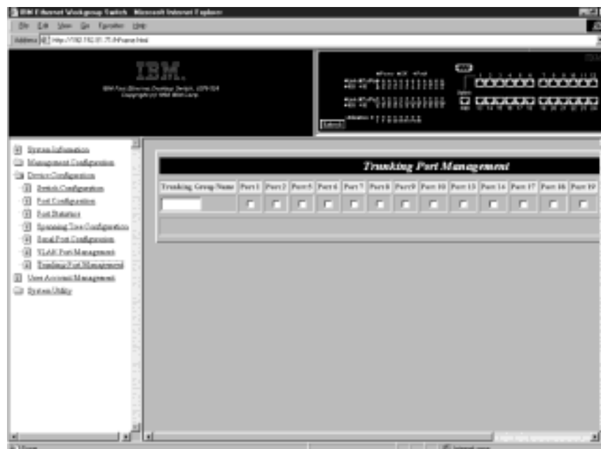
Figura 5-13. Panel Trunking Port Management
